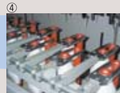
Forks simultaneously grasp full and empty bobbins
